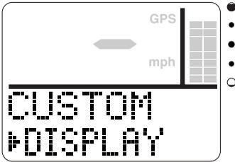
3. **(MODE)**: Press to switch between the setting function names (custom mode selection display).
