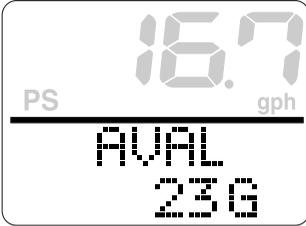
Resetting the AVAL (available: remaining fuel) and TTL (total fuel consumption) displays:
