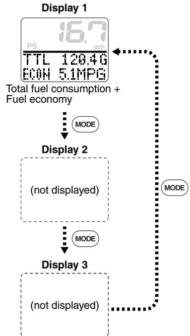
When the engine start switch is turned to OFF, the last display shown is shown first when the engine start switch is turned to ON again.
