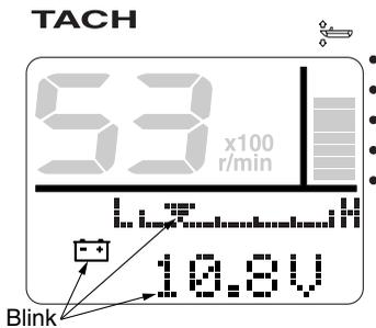
When the battery voltage decreases below the voltage that is required by the engine, the "LOW VOLTAGE" warning comes on.
