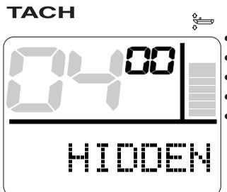
\* When the display configuration number "00" is selected, "HIDDEN" is shown and the display is not shown.
