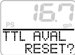
2. **SET** (1 second) or **SET** + **MODE** (1 second): To simultaneously reset the TTL and AVAL and return to the normal display.
