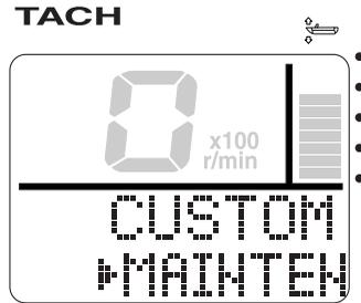
3. **(MODE)**: Press to switch between the setting function names (custom mode selection display).
