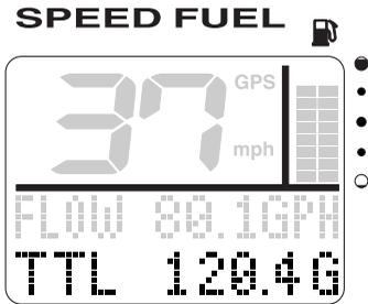
The TTL display cannot measure over 1,999 gallons or 1,999 liters. When exceeding 1,999 gallons or 1,999 liters of fuel, “▲” blinks in front of the numeric value to indicate an overflow.
