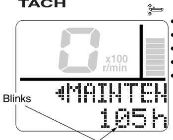
4. **SET** + **MODE** (1 second): To reset the elapsed time to "0h."
