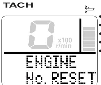
3. Turn the engine start switch to OFF. The engine number is reset after approximately 10 seconds.
