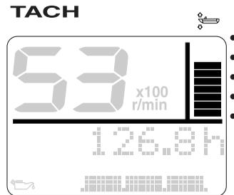
When the angle of the outboard motor exceeds the trim range, the top segment blinks.
