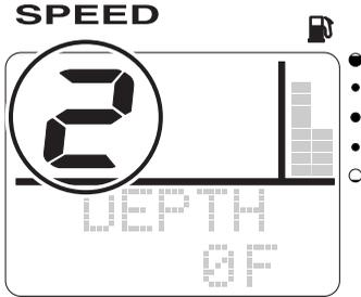
5. **SET**: To select the display configuration number (0–15) you want to change. The fuel level segments show the display configuration numbers. Press to switch between the display configuration numbers.
