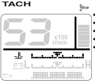
When the engine overheats, the cooling water/engine temperature indicator (
