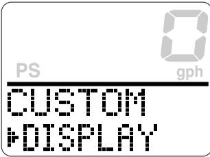
3. **MODE**: Press to switch between the setting function names (custom mode selection display).
