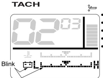
\* In the display example, the battery voltage level and the cooling water/engine temperature are shown.
