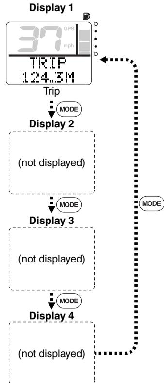
When the engine start switch is turned OFF, the last display shown is shown first when the engine start switch is turned to ON again.
