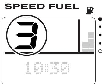
5. **(SET)**: To select the display configuration numbers (0–36) you want to change. The fuel level display segments (the left column represents the tens digit and the right column represents the ones digit) show the display configuration numbers. Press to switch between the display configuration numbers.
