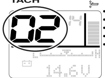
6. **SET**: To select the display format. Press to switch between each display format.
