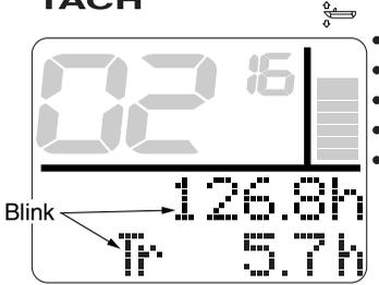
\* In the display example, the total operation hours and trip hours (Tr) are shown.
