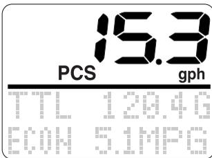
\* In the display example, the total fuel consumption of three outboard motors is shown.
