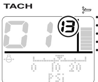
\* In the display example, display number 01 and display configuration number 13 are shown.
