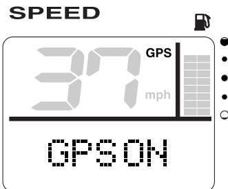
3. **SET** (1 second): To set the speed sensor and return to the normal display.
