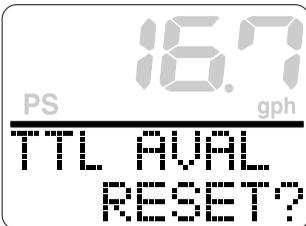
2. **SET** (1 second) or **SET** + **MODE** (1 second): To simultaneously reset the AVAL and TTL displays and return to the normal display.
