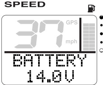
When the battery voltage decreases to 12 volts or less or increases to 16 volts or more the voltage value blinks.
