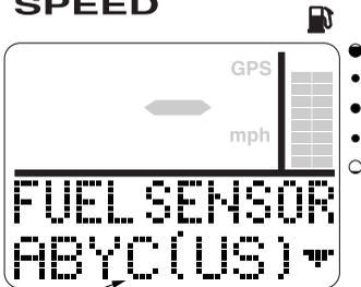
6. **SET** (1 second): To change the fuel sensor type and return to the custom mode selection display.
