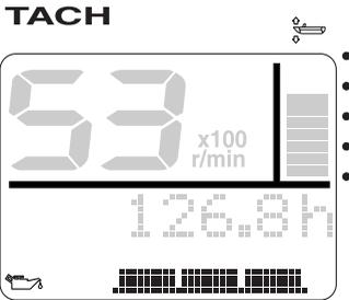
When the engine oil level is low, the oil level indicator (
