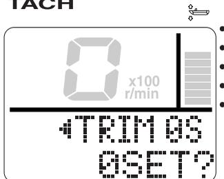
5. **(SET)** + **(MODE)** (1 second): To adjust the trim angle to zero using the current trim position as the standard value.
