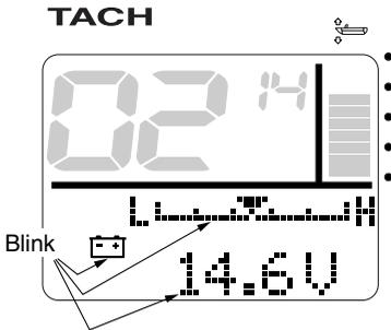
\* In the display example, the battery voltage value and battery voltage level are shown.
