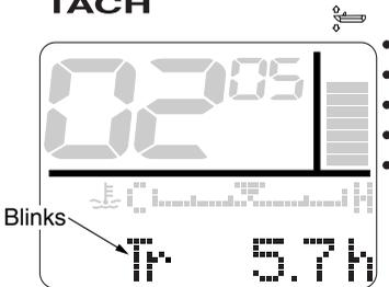
\* In the display example, the trip hours (Tr) and the cooling water/engine temperature are shown.
