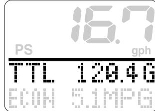
The TTL display cannot measure over 1,999 gallons or 1,999 liters. When exceeding 1,999 gallons or 1,999 liters of fuel, “▲” blinks in front of the numeric value to indicate an overflow.
