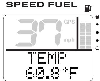
**NOTE:** You can select to show Fahrenheit (°F) or Celsius (°C) on the TEMP display. To change the displayed unit, see “UNIT (setting displayed units)” in “Changing settings (custom mode).”
