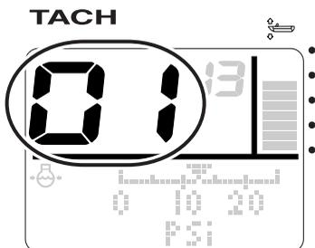
6. **SET**: To select the display configuration numbers (00–16) you want to change. The last two digits in the tachometer display show the display configuration numbers. Press to switch between the display configuration numbers.
