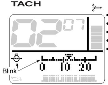
\* In the display example, the cooling water pressure level (with scale) is shown.
