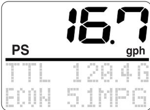
\* In the display example, the total fuel consumption of two outboard motors is shown.
