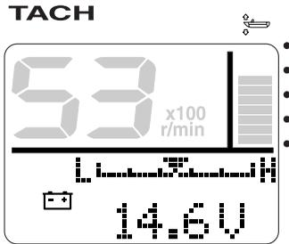
When the battery voltage decreases to 12 volts or less or increases to 16 volts or more the battery voltage indicator (
