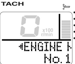
6. **SET** (1 second): To change the corresponding engine and return to the custom mode selection display.
