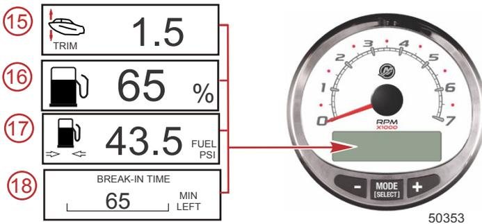
15. **Power Trim Angle/Water Pressure:** Displays the trim angle of the engine and cooling system water pressure.
