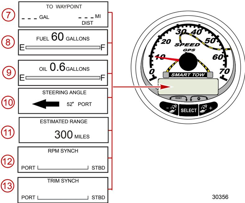
7. **To Waypoint:** Displays the amount of fuel to the waypoint and the distance to the waypoint. A GPS unit with waypoints capability must be installed to display the distance to the waypoint.
