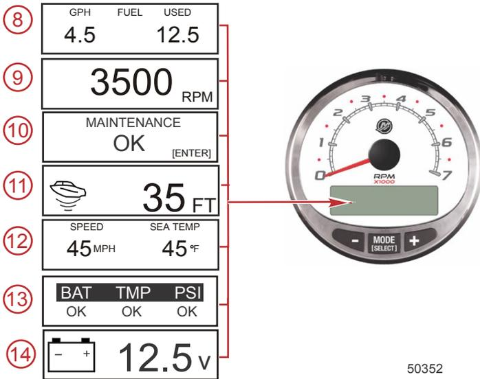
8. **Fuel Flow:** Displays fuel use in gallons or liters per hour, and overall amount of fuel used.
