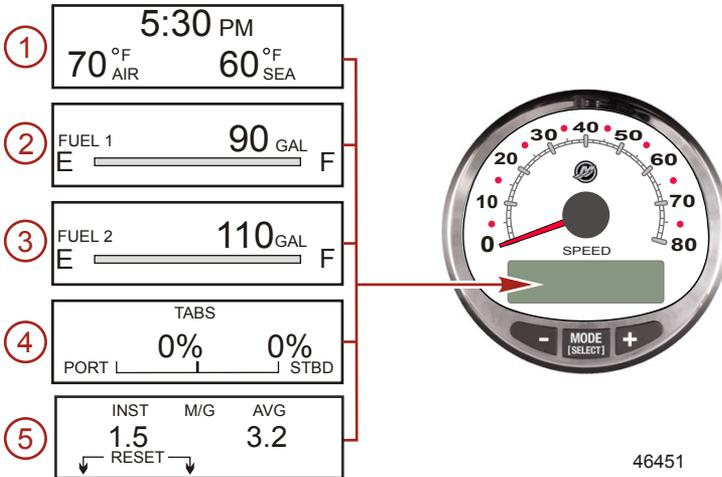
When the ignition is turned on, the speedometer will show the last screen that was displayed before the ignition was turned off. Press "MODE/SELECT" to change display screens. Revert back to the previous screen by pressing and holding "MODE/SELECT" for two seconds.
