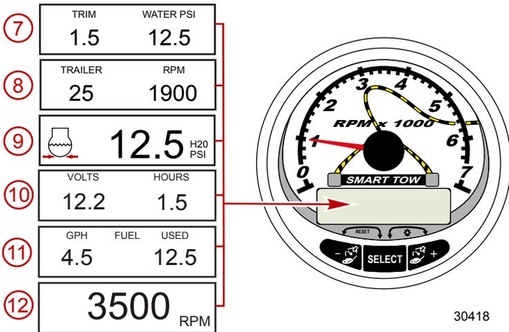
7. **Trim Position/Water Pressure:** Displays the trim angle of the engine or drive system and cooling system water pressure.
