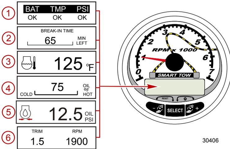
When the ignition is turned on, the tachometer will display the last screen that was displayed before the ignition was turned off. Press "SELECT" to change display screens. Revert back to the previous screen by pressing and holding "SELECT" for two seconds.
