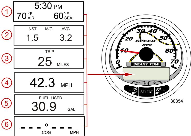
When the ignition is turned on, the speedometer will show the last screen that was displayed before the ignition was turned off. Press "SELECT" to change display screens. Revert back to the previous screen by pressing and holding "SELECT" for two seconds.
