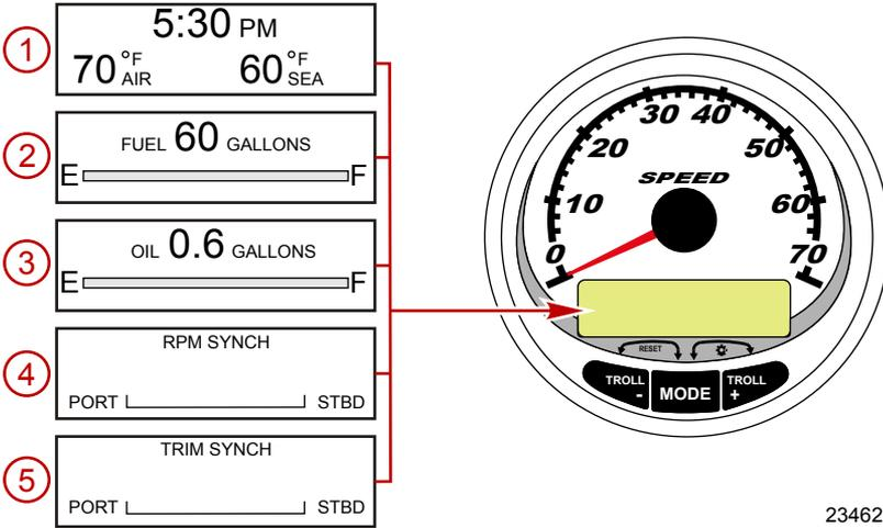
When the ignition is turned on, the speedometer will show the last screen that was displayed before the ignition was turned off. Press "MODE/SELECT" to change display screens. Revert back to the previous screen by pressing and holding "MODE/SELECT" for two seconds.
