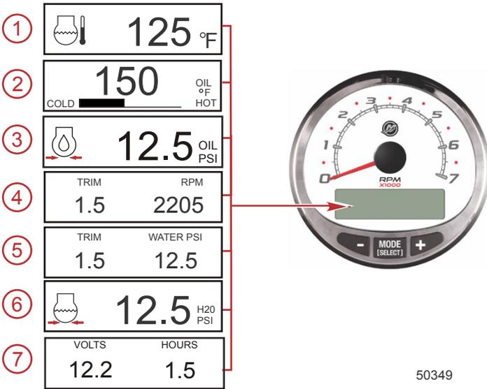
1. **Temperature:** Displays the engine coolant temperature.
