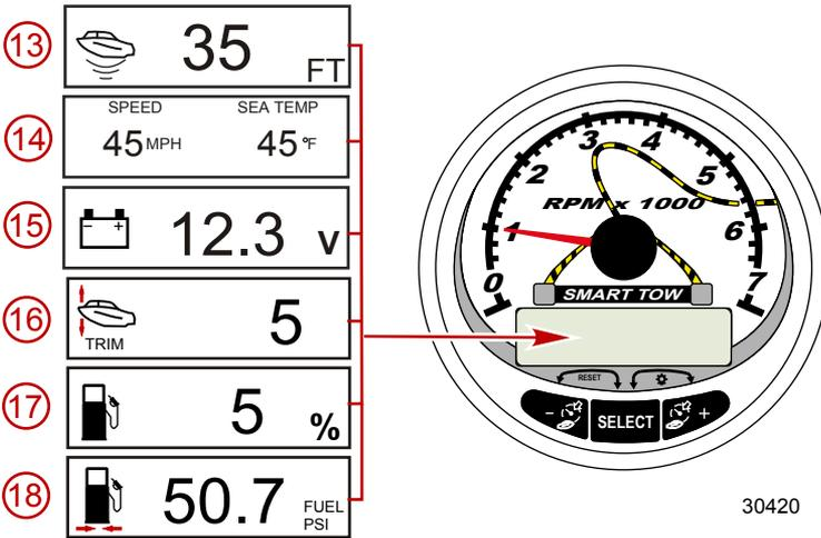
13. **Water Depth:** Displays the depth of water under the transducer if connected. The water depth screen can be turned on or off in CAL 1 calibration. The alarm can be set to trigger whenever the boat moves into water shallower than the alarm level. Refer to CAL 2 calibration for water depth alarm and offset settings.
