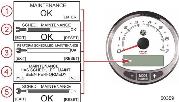
2. The scheduled maintenance screen displays a bar graph indicating the estimated time remaining on the scheduled maintenance cycle. Press "EXIT" to return to the previous screen or "RESET" after the scheduled maintenance has been performed.
