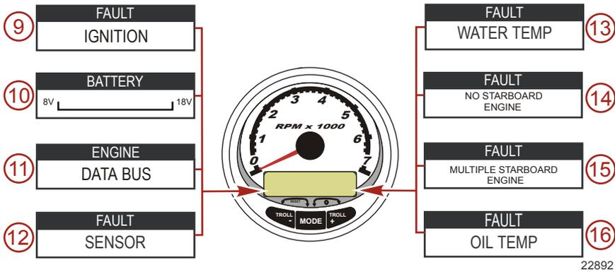
9. **FAULT - IGNITION:** A problem has developed in the ignition system.
