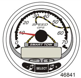
The second generation of the SmartCraft speedometer known as Smart Tow. The external appearance changed with a rope on the gauge face and the buttons show a symbol for cruise control. Digital control of the engine above trolling RPM is available. The SmartCraft GPS puck is introduced and can be connected directly to the gauge harness or a junction box.
