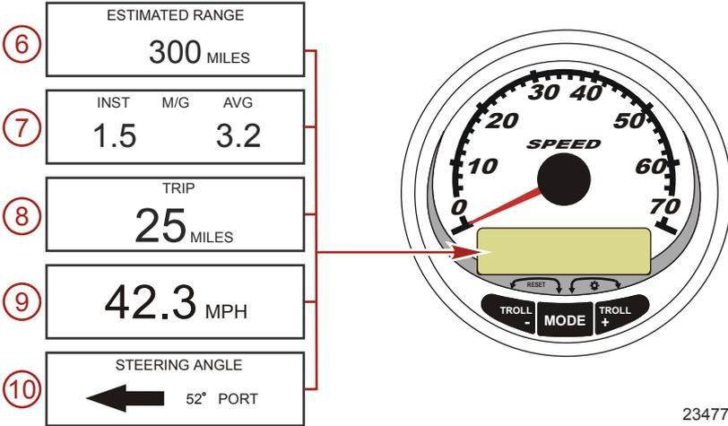
6. **Range:** The estimated range is based on boat speed, fuel consumption, and fuel remaining in the tank. The numbers displayed are an estimate of the distance you can travel with the remaining fuel. Speed input required (paddle wheel, pitot pressure or GPS).
